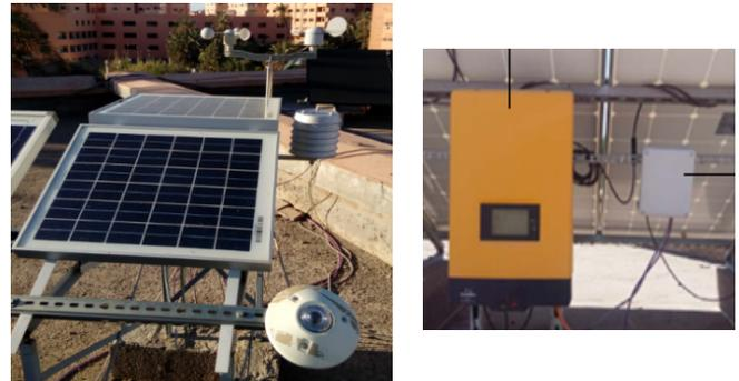
Fig. 2. Weather station (left) and electrical data acquisition system nearby the inverter (right).
