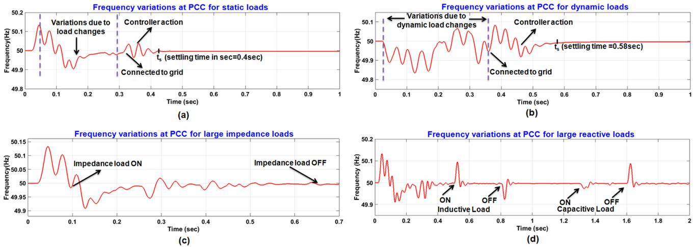
**Fig. 8.** Frequency response of minigrad system under grid connected mode for a) Static loads b) Dynamic loads c) Large impedance loads d) Large reactive loads.
