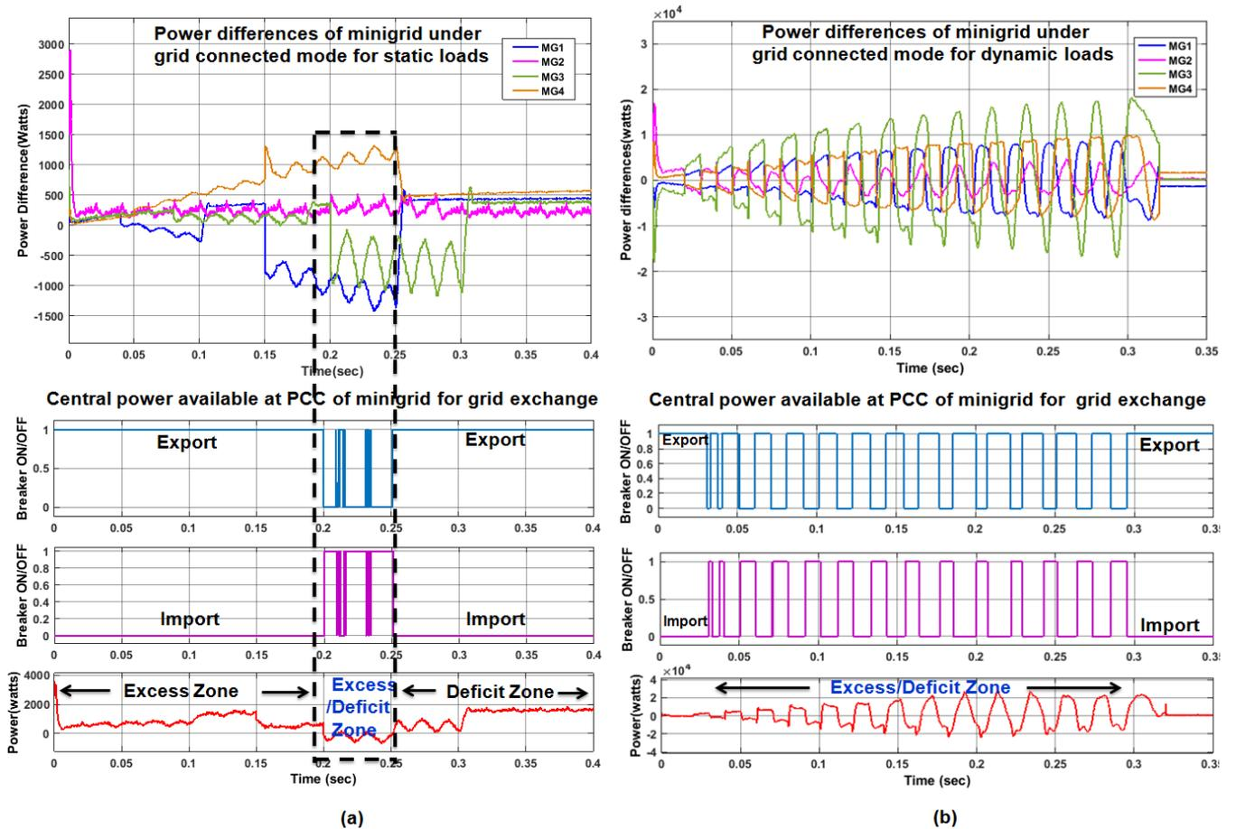
**Fig. 9.** Minigrad power differences and total power available at PCC for exchange for a) Static loads b) Dynamic loads.
