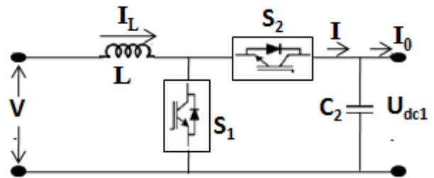
Fig. 2. Equivalent circuit of boost converter
