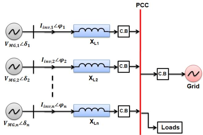
Fig. 4. Single line diagram of interconnected microgrids
