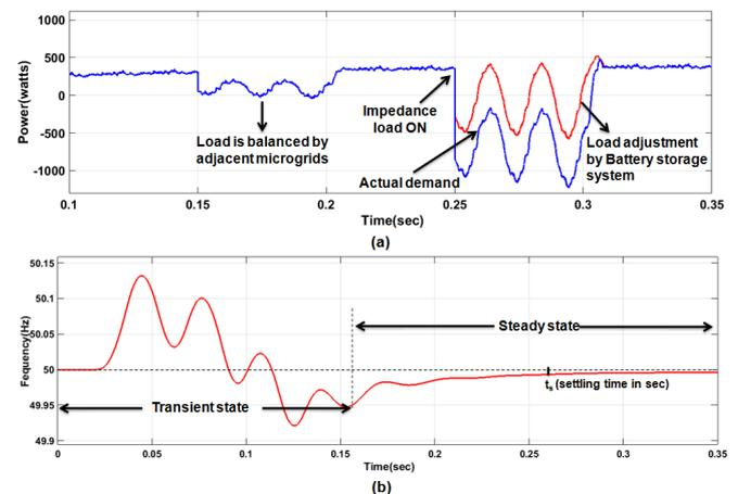
Fig. 7. a) Demand response of minigrid b) Frequency response of minigrid in islanded mode.
