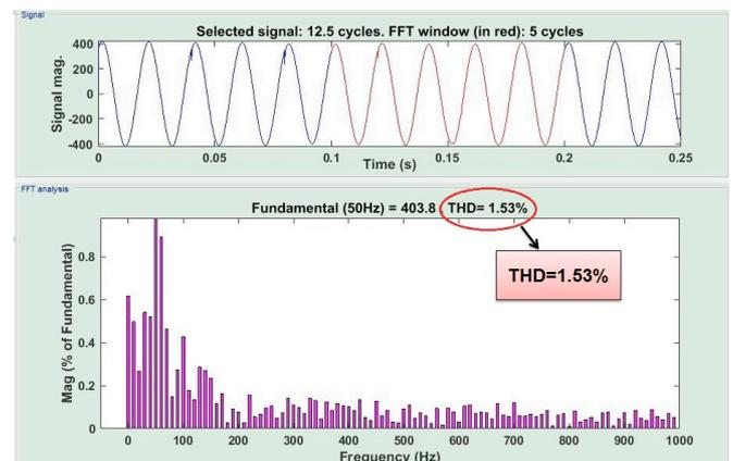
**Fig. 11.** FFT analysis for harmonic distortion in the minigrid
