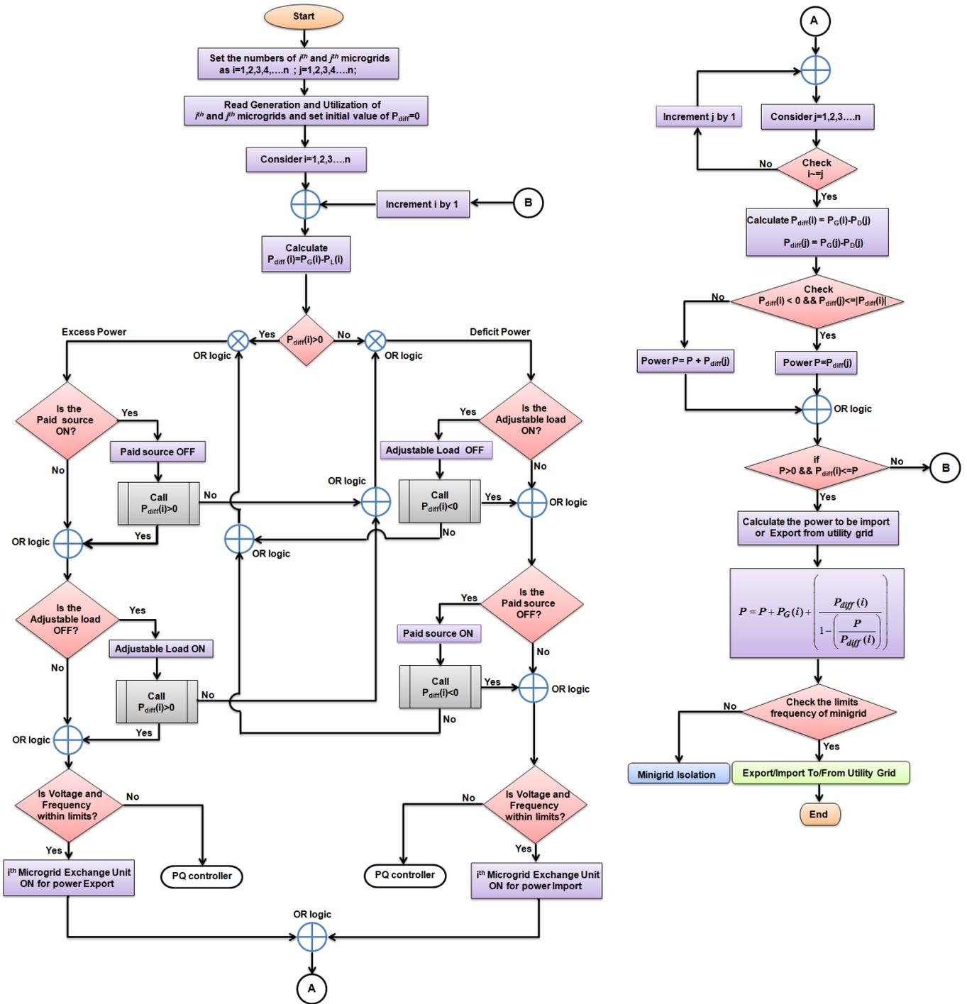
Fig. 5. Flow chart of proposed controller modelled in MATLAB/Simulink
