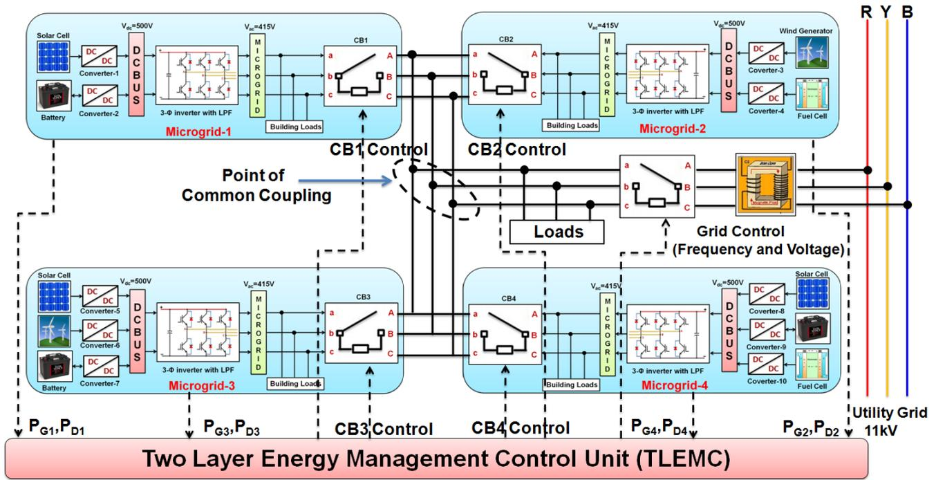
Fig. 1. General architecture of minigrid system
