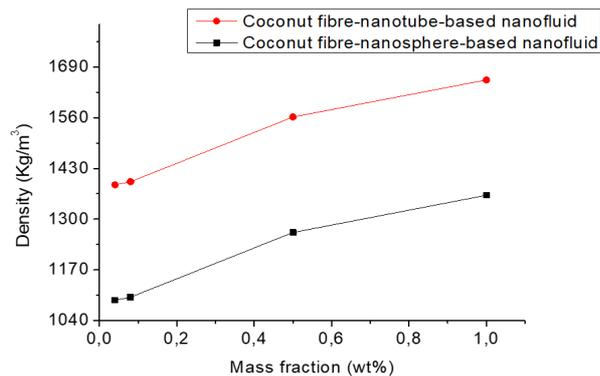
Fig. 8. Weight fraction variation of densities from CF nanotube and CF nanosphere-based nanofluids at 0.04 wt%
