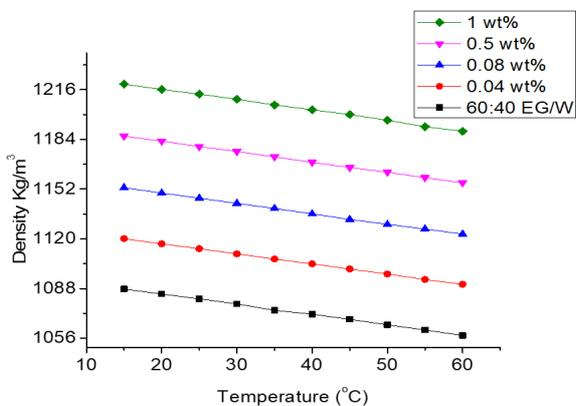
Fig. 5. Density of CF nanosphere-based nanofluid
