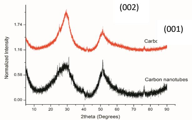
**Fig. 3.** X-ray Diffractogram of CF carbon nanosphere and CF carbon nanotubes
