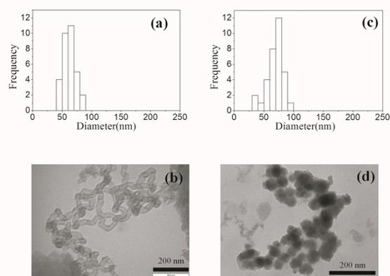
**Fig. 1.** Particle size distribution and TEM images of CF (a) carbon nanotubes and (b) carbon nanospheres
