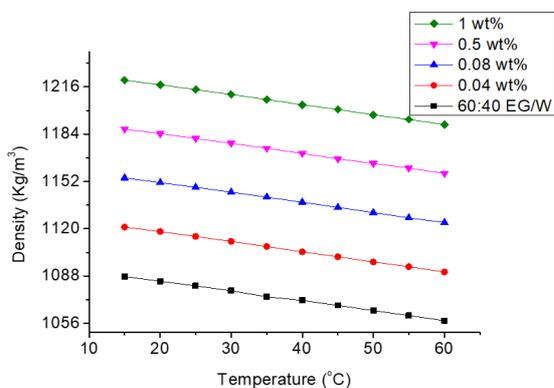
Fig. 6. Density of CF nanotube-based nanofluid
