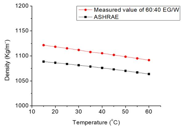
**Fig. 4.** Measured value of 60:40 EG/W and ASHRAE value of 60:40 EG/W
