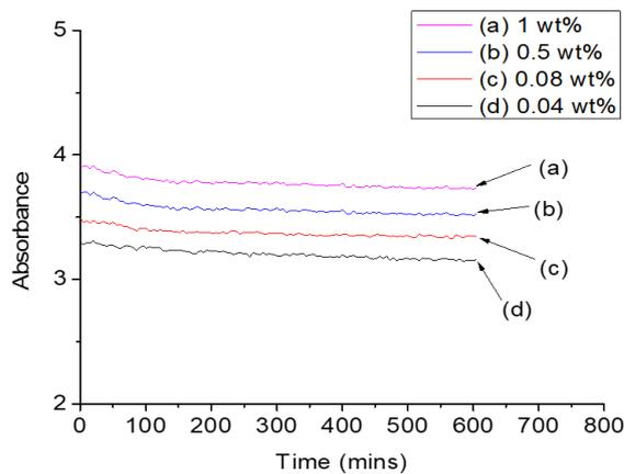
**Fig. 1.** Stability test for CF based nanosphere-nanofluid using UV Spectroscopy at a constant temperature for 700 minutes
