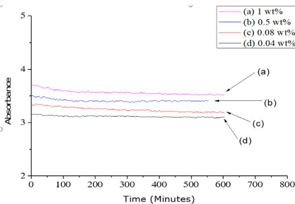
**Fig. 2.** Stability test for CF based nanotubes-nanofluids using UV Spectroscopy at a constant temperature for 700 minutes
