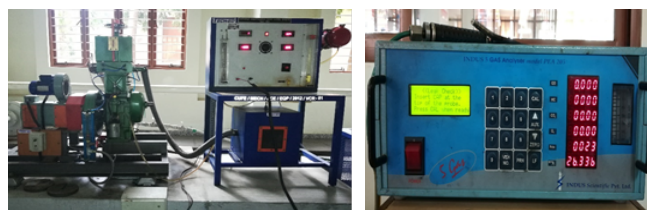
Fig. 5. Engine test rig and 5-gas analyzer
