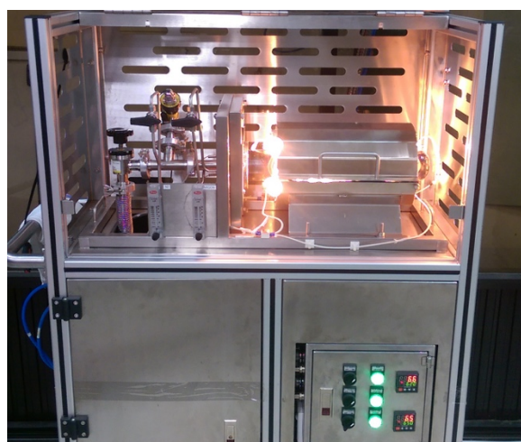
Fig. 2. CSS equipment used for CdTe film deposition.
