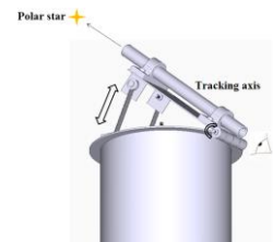
Figure 29. The orientation of the tracking axis towards the pole star.
