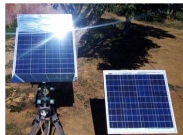
Figure 36. The solar panel on the left in the tracking mode, the one on the right in the fixed mode.
