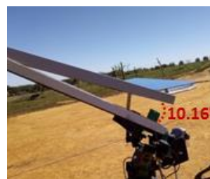
Figure 38. The tilt of the photovoltaic panel for the test of the bottom mirror.
