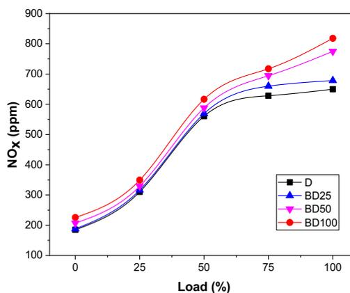
**Fig. 7.** Effect of engine load on NO<sub>x</sub> using CI engine in different test fuels
