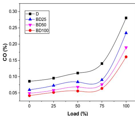
**Fig. 6.** Effect of engine load on CO emission using CI engine in different test fuels
