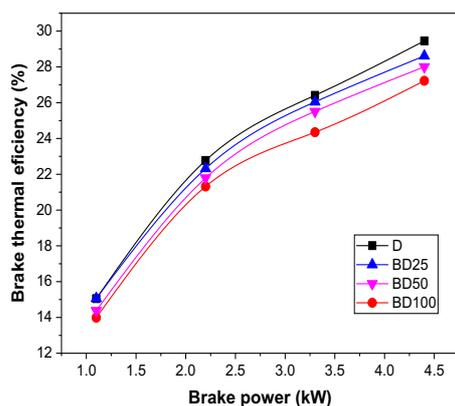
Fig. 3. Effect of engine load on BTE using CI engine in different test fuels
