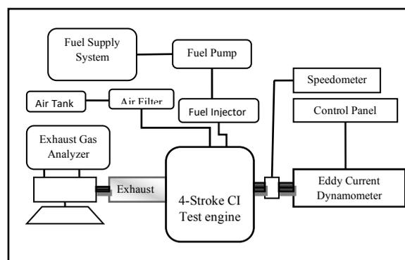
**Fig. 2. Schematic diagram of 4S-CI test-setup**
