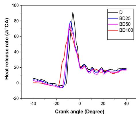
Fig. 11. Heat release rate due to different test fuels
