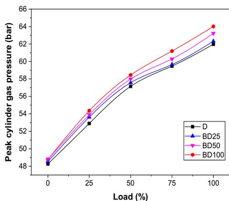
Fig. 12. Peak cylinder gas pressure due to different test fuels
