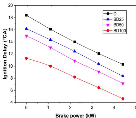
Fig. 9. Effect of engine load on ignition delay period due to different test fuels
