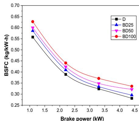
Fig. 4. Effect of engine load on BSFC using CI engine in different test fuels
