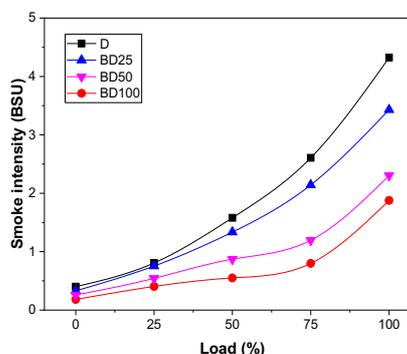
**Fig. 8.** Effect of engine load on smoke intensity emission using CI engine in different test fuels
