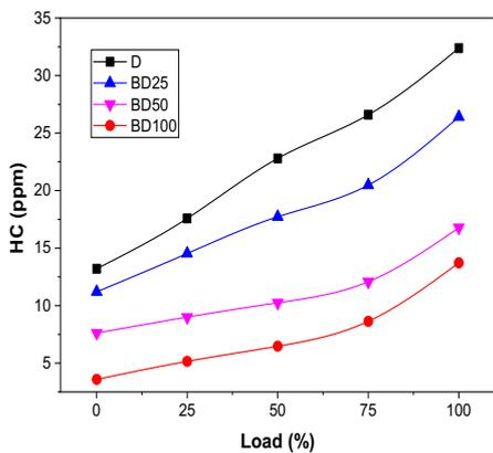
**Fig. 5.** Effect of engine load on HC emission using CI engine in different test fuels
