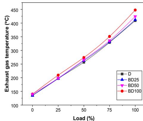
Fig. 10. Effect of engine load on exhaust gas temperature variation due to different test fuels
