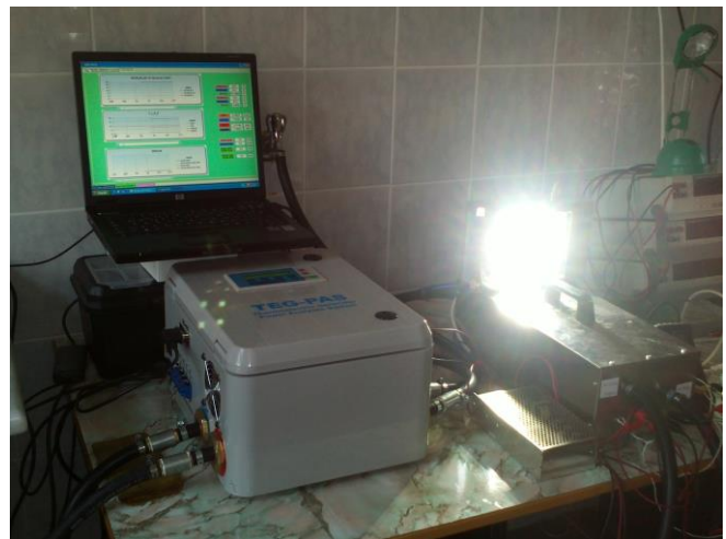
Fig. 9. A portable geothermal TEG of 100W
