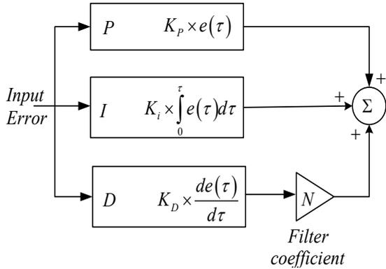
**Fig. 2.** Controller applied for the system considered
