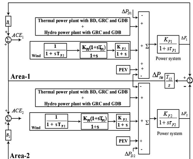
**Fig. 7.** Modified system configuration by integration of wind turbine to the existing system.
