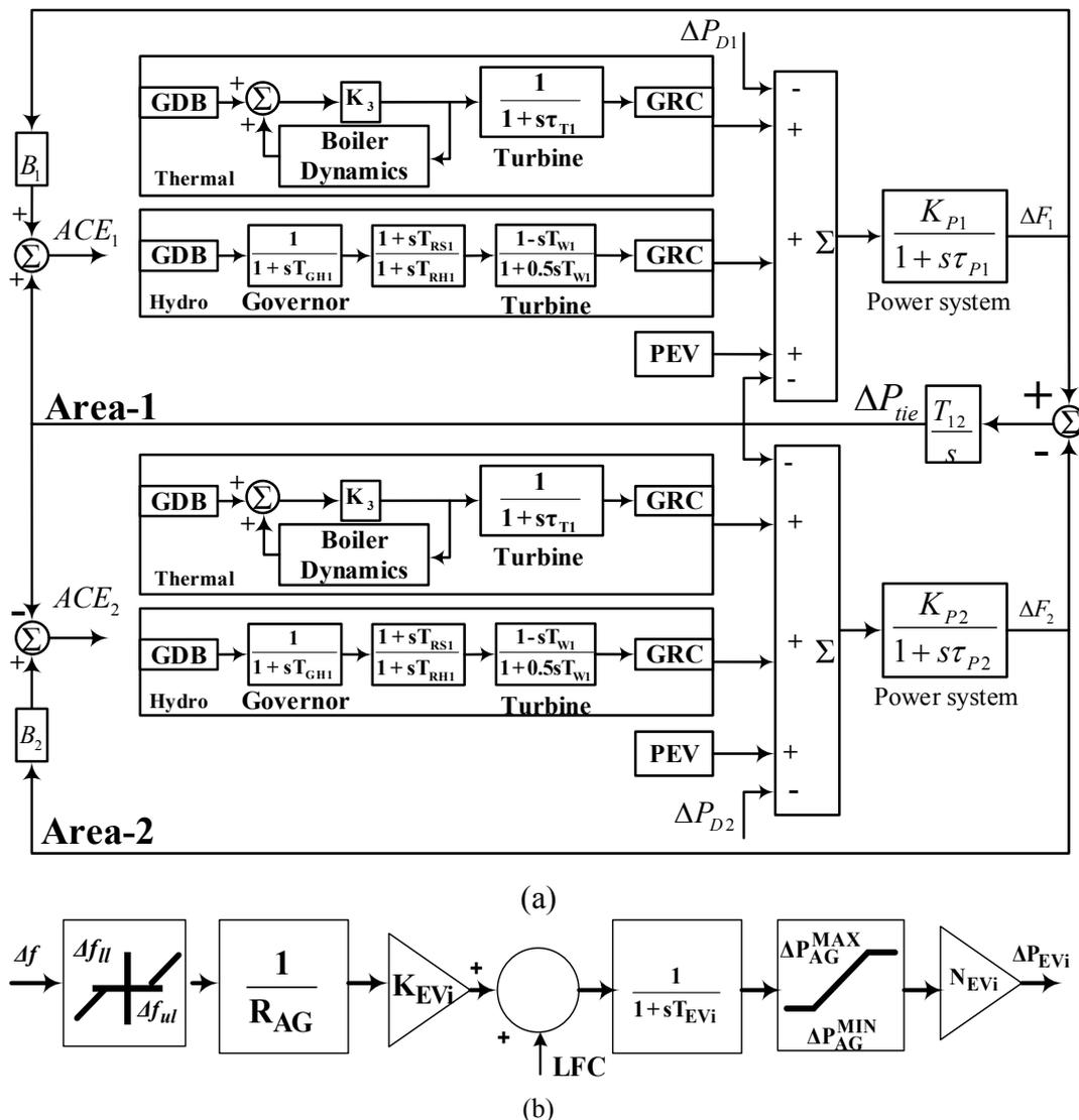
Fig. 1. (a) The 2-area hydro-thermal system transfer function model, (b) Transfer function model of PEV
