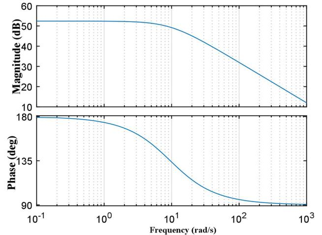
**Fig. 9.** Magnitude and Phase plot of the test system
