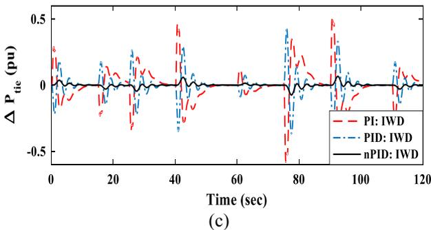
Fig. 6. System response for Dynamic load variation.
